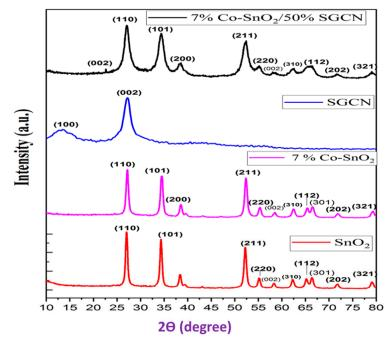
Figure 1. XRD pattern of SnO<sub>2</sub>, 7%Co-SnO<sub>2</sub>, SGCN, and 7%Co-SnO<sub>2</sub>/50% SGCN.
