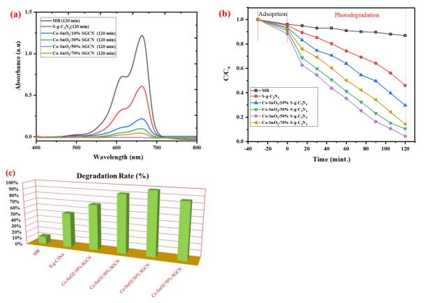
Figure 7. Degradation contours (a) Degradation rate (b) % Degradation of MB (c) by Co-SnO<sub>2</sub>/SGCN.
