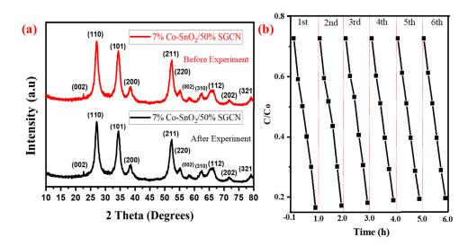
**Figure 9.** The stability and recyclability of the photocatalyst (**a**). X-ray diffraction patterns of the Co-SnO<sub>2</sub>/50% SGCN NCs before the experiment and after the 6th cycle (**b**).
