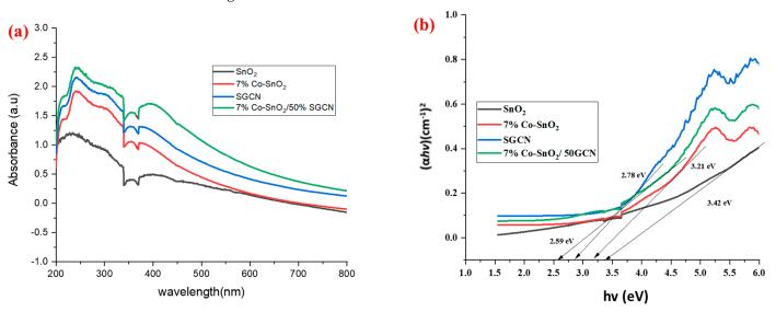
Figure 5. Absorption spectra (a) and bandgap of SnO<sub>2</sub>, 7% Co-SnO<sub>2</sub>, and 7% Co-SnO<sub>2</sub>/50% SGCN (b).
