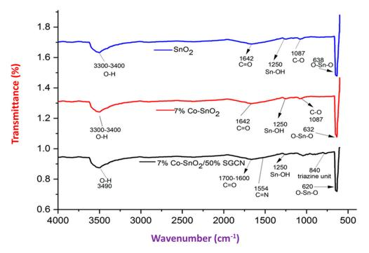
Figure 4. FTIR spectra of SnO<sub>2</sub>, 7% Co-SnO<sub>2</sub> and 7% Co-SnO<sub>2</sub>/50% SGCN.
