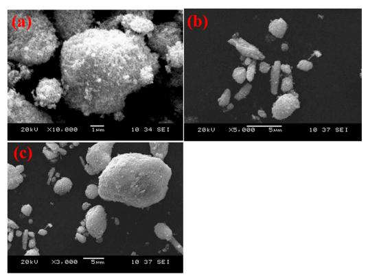
Figure 3. SEM images of SnO<sub>2</sub> (a), Co-SnO<sub>2</sub> NPs (b), and Co-SnO<sub>2</sub>/SGCN NCs (c).
