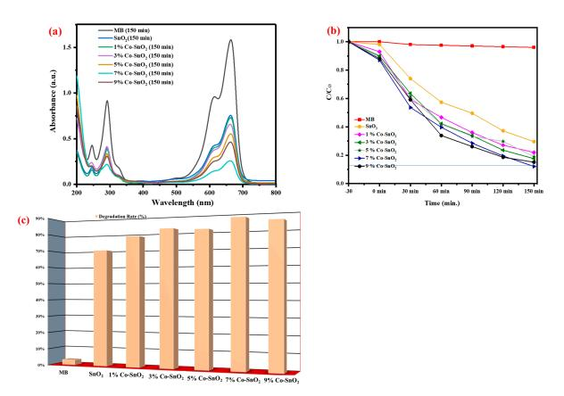
**Figure 6.** Degradation contours (a) Degradation rate (b) % Degradation of MB (c) by  $SnO_2$  and  $Co-SnO_2$  NPs.
