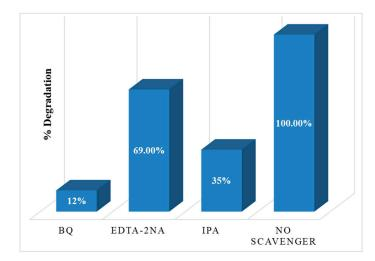
Figure 8. Effect of radical scavengers in the catalytic degradation of MB with Co-SnO<sub>2</sub>/50% SGCN.
