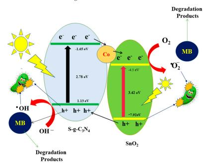
**Figure 11.** An illustration of the catalytic degradation mechanism of MB under sunlight over the  $Co-SnO_2/S-g-C_3N_4$  NCs.
