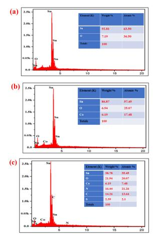
Figure 2. EDX images of  $SnO_2$  (a), Co- $SnO_2$  NPs (b), and Co- $SnO_2/SGCN$  NCs (c).
