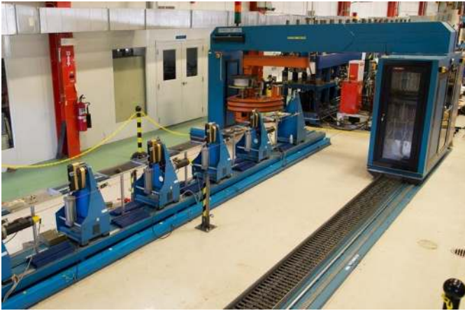
Fig. 1a. Spirex Selva coil winding machine
