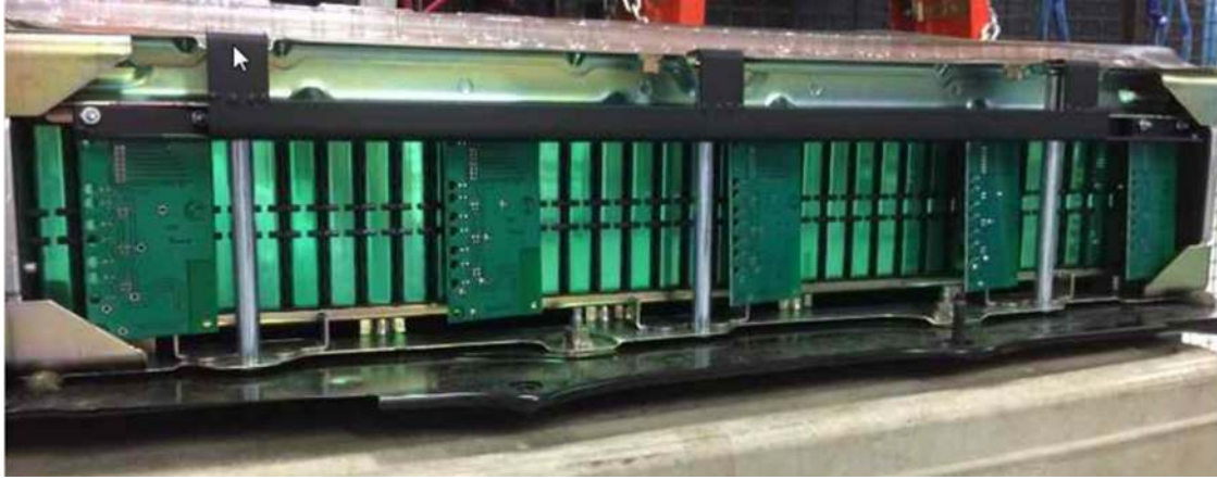
Fig. 7 A rail (shown in black) was designed to hold the electronics needed for the sensors. The boards were oriented to allow flow through to the cells.
