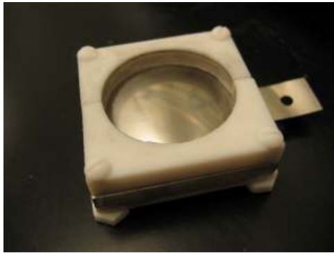
Fig. 13. Electrode assembly for electrophoretic deposition of the optimized initial shape.
