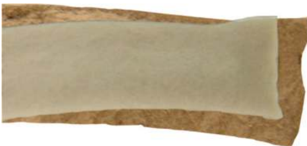
Fig. 14. Comparison between a green specimen and a sintered specimen.
