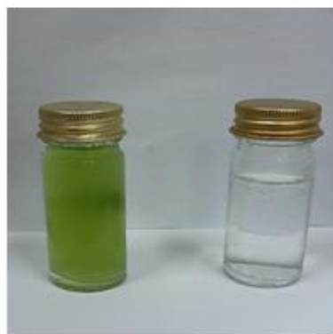
Fig. 5: Picture of before and after filtration of Nannochloropsis sp. solution by the PES modified membranes.
