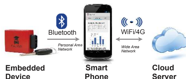
Figure 1. An example MGC application distributes logic and user interaction across embedded device, mobile phone and a cloud server.
