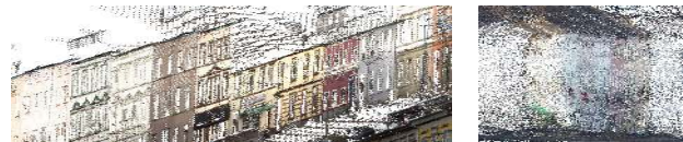
Figure 1. Facades in a terrestrial laser scanning point cloud (left) vs. facades in a photogrammetric point cloud (right)
