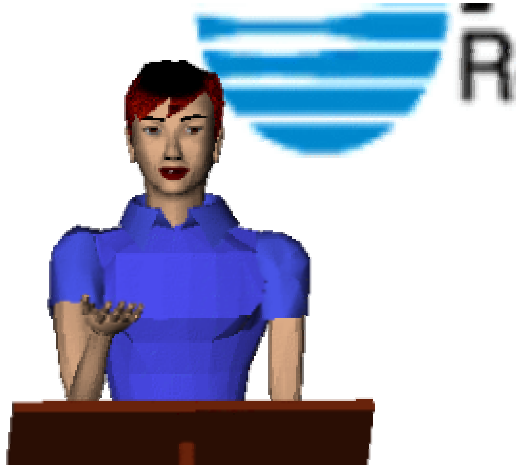
Figure 6: Using MPEG-4 face animation tools, face and body of this model can be downloaded and efficiently animated by the encoder that downloads the model to the decoder.
