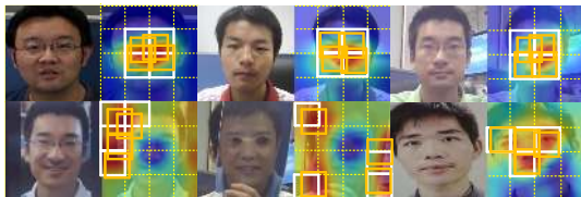
Figure 6. The attended local regions by RAM on live faces (top) and spoofer faces (bottom), respectively. Please notice that the attended regions are consistently in the center on live face images, while are diverse on spoofer face images, indicating cues such as borders. Best viewed in color.
