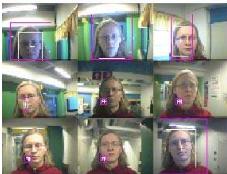
Fig. 33. Face tracking with fixed histogram. The magenta box shows the search area while the white box and cross display the face localization.
