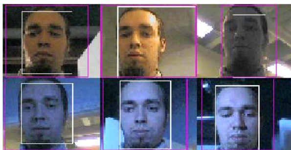
Fig. 31. A few selected frames from the skin locus based adaptive face tracking for a video taken by an Alaris webcam. White boxes visualize localization of the bounding box and magenta boxes show the search area.
