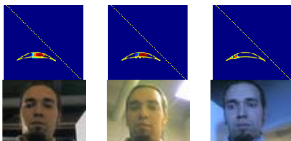
Fig. 29. Behavior of the ratiohistogram. The upper image row shows how the ratiohistogram of a face image is affected by the colour appearance of skin. The skin locus is visualized with two straight lines. The reddish colour in the upper row means high values whereas the blue indicates low values.
