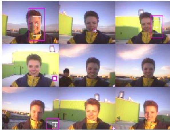
Fig. 35. Adaptive tracking using an elliptical constraint. The magenta box shows the search area while the white box and cross display the face localization.
