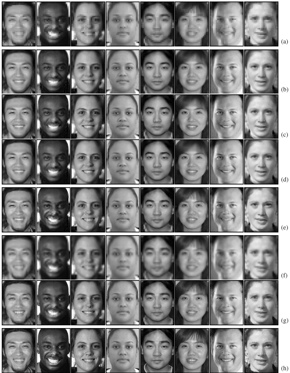
Figure 7. Comparison of different algorithms. (a) Input low-res face images. (b) Reconstruction by global face model (soft constraint). (c) Reconstructed by combining the global with the local face model, obtained from the nonparametric Markov network. Many local facial details are added from (b) to (c), e.g. highlights in eyeballs, teeth. (d) Results after post-processing by smart bilateral filtering. Some noise and ghosting artifacts caused by PCA reconstruction are removed. (e) Hallucinated results by hard constraint. We also compare our algorithm with others. (f) Bicubic interpolation. (g) Freeman et. al. [14]’s approach, adapted to be inhomogeneous to meet [1]. Although facial detailed features can be reconstructed locally, the global facial features are in general lost via this approach. (h) Original high-res images.
