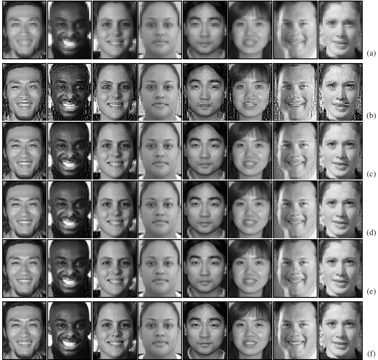
Figure 6. Experimental results on reconstructing the global face I_H^g using the hard constraint. (a) Input 24 \times 32 low-res images. From (b) to (e) are global faces inferred using the hard constraint with different eigenspace dimensions. (b) r = 1000 , (c) r = 1500 , (d) r = 2000 , (e) r = 2500 . (f) Original 96 \times 128 high-res images. With fewer eigenvectors the reconstructions were noisy, because there is not much freedom to maximize the probability in the eigenspace given the low-res constraint. With more eigenvectors, however, most of the errors diminish. In (b) and (c) we may observe similar ghosting effect to the reconstruction using the soft-constraint.
