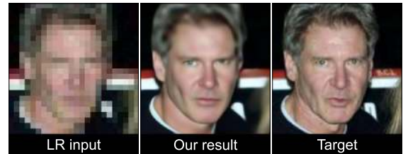
Fig. 1. Face hallucination results generated with the C-SRIP model. The figure shows (from left to right): a 24 \times 24 low-resolution (LR) input face image, the 8\times super-resolved (SR) image, and the high-resolution (HR) ground truth. Note that C-SRIP is able to ensure visually convincing super-resolution results.
