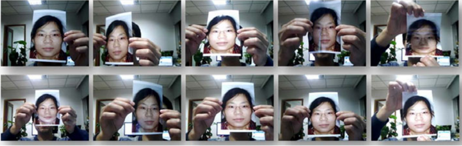
Fig. 4. Illustration of different photo-attacks (from left to right) : (1) move the photo horizontally, vertically, back and front; (2) rotate the photo in depth along the vertical axis; (3) the same as (2) but along the horizontal axis; (4) bend the photo inward and outward along the vertical axis; (5) the same as (4) but along the horizontal axis
