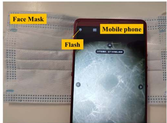
Fig. 2. Scenario of the portable detection device's working. While the device is on work, the flash must meet the condition that the flash is always "on" to provide enough light.
