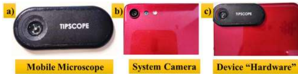
Fig. 1. The overview of the portable detection device's "Hardware". The "Hardware" is composed of a mobile microscope, a phone with available system camera, etc. Specifically, a) and b) represent the mobile microscope and system camera, respectively; and c) shows the final removable device mainly assembled by a) and b).
