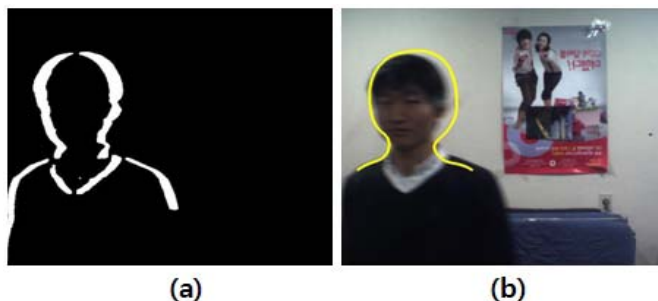
Figure 2. A lag problem of head and shoulder detection. (a) and (b) show the binarized frame difference image and corresponding head and shoulder countour, respectively.
