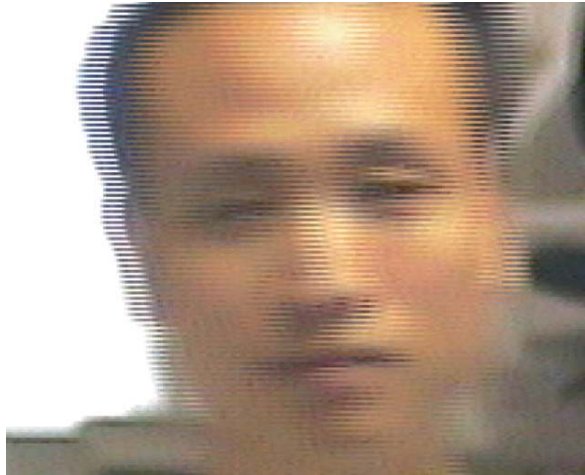
Fig. 6.3 The image captured by CCTV camera with interlace problem
