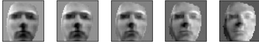
Fig. 5. Learning complex illumination effects: Shown is the variation along the 1st mode of a single PPCA space in our SIM mixture model. Cast shadows (e.g. from the nose) and the locations of specularities (on the nose and above the eyes) are learnt as the illumination source moves from directly overhead to side-overhead.
