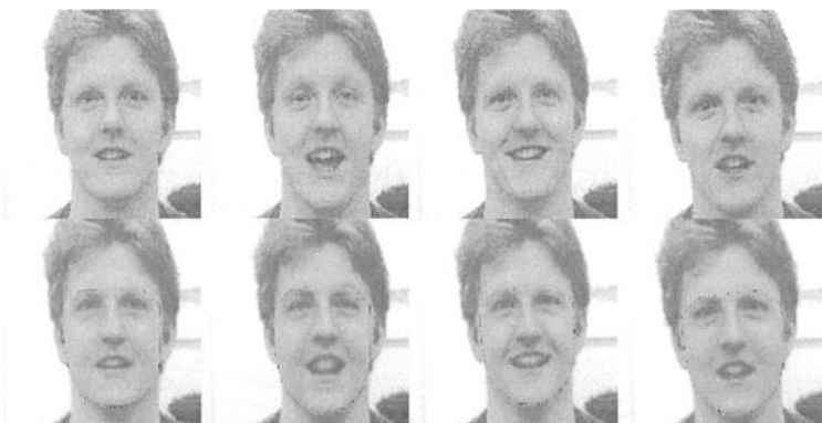
Fig. 7. Tracking and identifying a face. Original frames are shown on the top row, reconstruction on the bottom.
