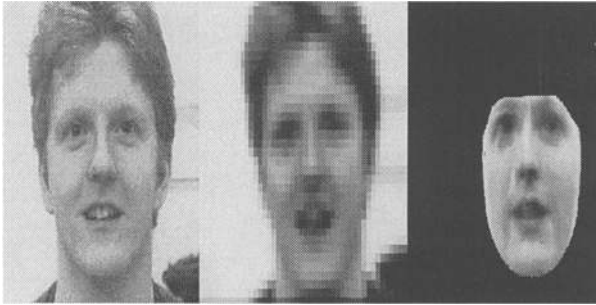
Fig. 12. Synthesising a high-res face from a low-res sequence. Left hand image: an original frame from sequence. Centre image: frame from deliberately blurred sequence. Right hand image: final reconstruction from low-res sequence
