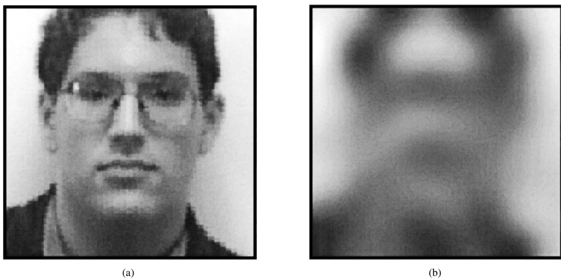
Figure 4. Effect of reconstructing a 128 \times 128 image using only 64 DCT coefficients: (a) original (b) reconstructed.
