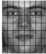
Fig. 2. An example of face image divided into 7 \times 8 regions with size of 20 \times 15
