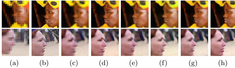
Fig. 4. Comparisons of different losses for the super-resolution. Columns: (a) Unaligned LR inputs. (b) Original HR images. (c) \mathcal{L}_p . (d) \mathcal{L}_p + \mathcal{L}_f . (e) \mathcal{L}_p + \mathcal{L}_f + \mathcal{L}_U . (f) \mathcal{L}_p + \mathcal{L}_h . (g) \mathcal{L}_p + \mathcal{L}_f + \mathcal{L}_h . (h) \mathcal{L}_p + \mathcal{L}_f + \mathcal{L}_U + \mathcal{L}_h . For simplicity, we omit the trade-off weights.
