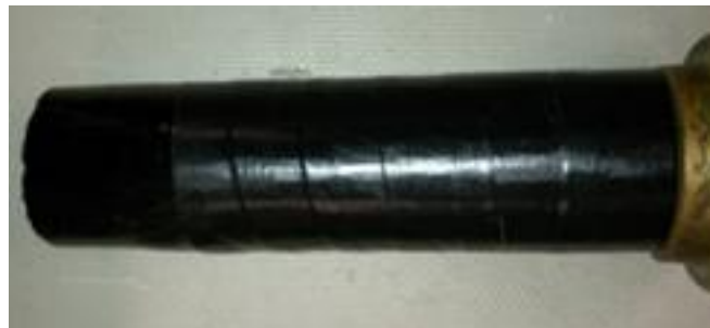
(b) Flexible ferrite around the shaft for magnetic shielding
