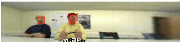
Figure 7. Initialisation of particle tracker with the face detection algorithm.
