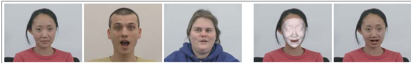
Figure 1: Face Transfer with multilinear models gives animators decoupled control over facial attributes such as identity, expression, and viseme. In this example, we combine pose and identity from the first frame, surprised expression from the second, and a viseme (mouth articulation for a sound midway between "oo" and "ee") from the third. The resulting composite is blended back into the original frame.
