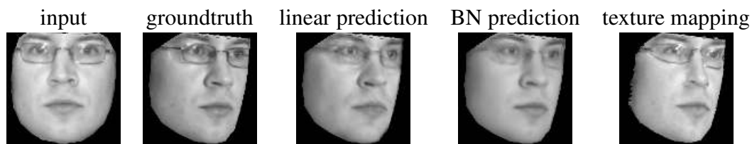
Figure 4.3: Results showing specularities on glasses. The texture mapping prediction gives fake reflections on glasses. And the shape of the glasses is also predicted incorrectly due to the difference in the 3D structures between this subject and the general face model.
