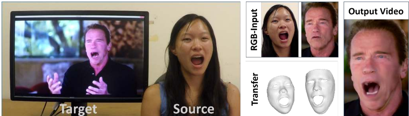
Proposed online reenactment setup: a monocular target video sequence (e.g., from Youtube) is reenacted based on the expressions of a source actor who is recorded live with a commodity webcam.
