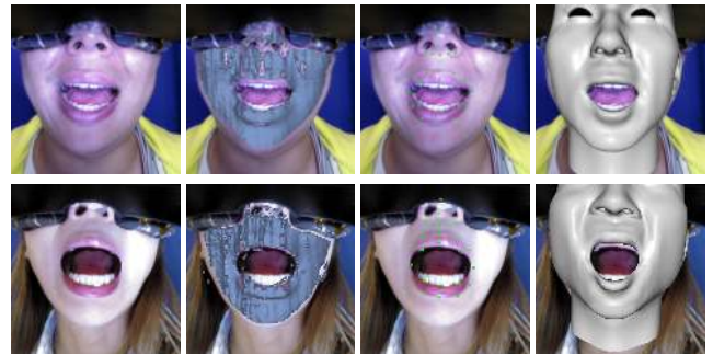
Figure 8: Optical input of our system. From left to right: RGB input; depth input; extracted 2D lip feature points; output mesh overlaid with the RGB input.
