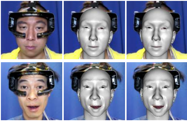
Figure 14: Comparison between our approach and state of the art real-time facial performance capture method. From left to right: input; [Li et al. 2013]; our result.
