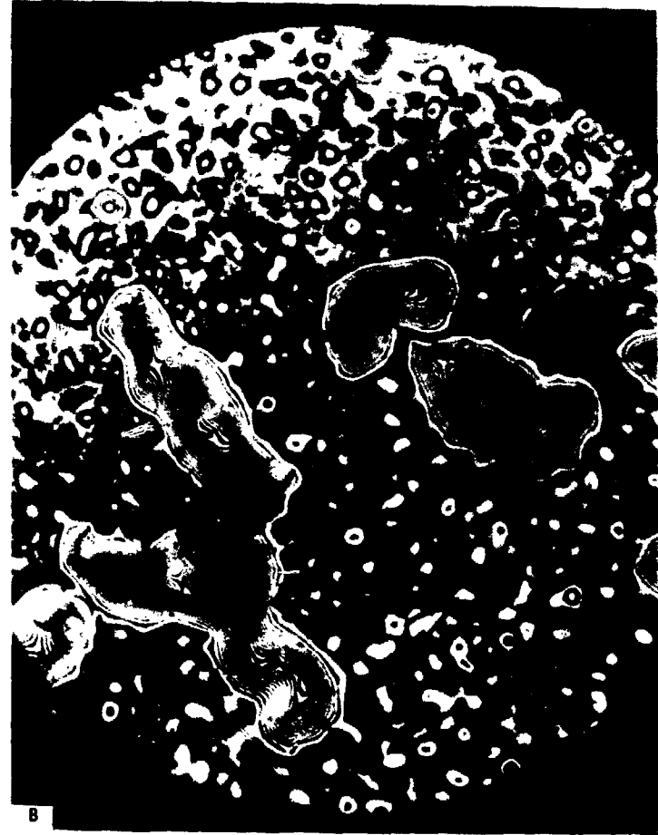
Fig. 8: Microinterferograms of delayed blistering of boron carbide B_4C , Ceralloy 546, H^+ (140 keV), 228 mC/cm 2 , contour interval 0.27 \mu . A. Diameter of circle 1.82 mm; B. Left side of previous picture at higher magnification, diameter of circle 0.72 mm. The large blisters did not appear until several months after bombardment.
