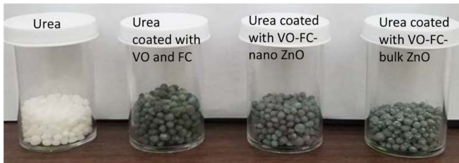
FIGURE 2 | Urea granules, and urea granules coated with vegetable oil (VO) and food coloring (FC), without and with, ZnO nano or bulk powders.
