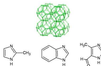
Fig. 1 Schematic drawing of the frameworks of sodalite and imidazolate linkers methylimidazole (ZIF-8), benzimidazole (ZIF-7), 4-methyl-5-imidazolecarboxaldehyde (SIM-1).
