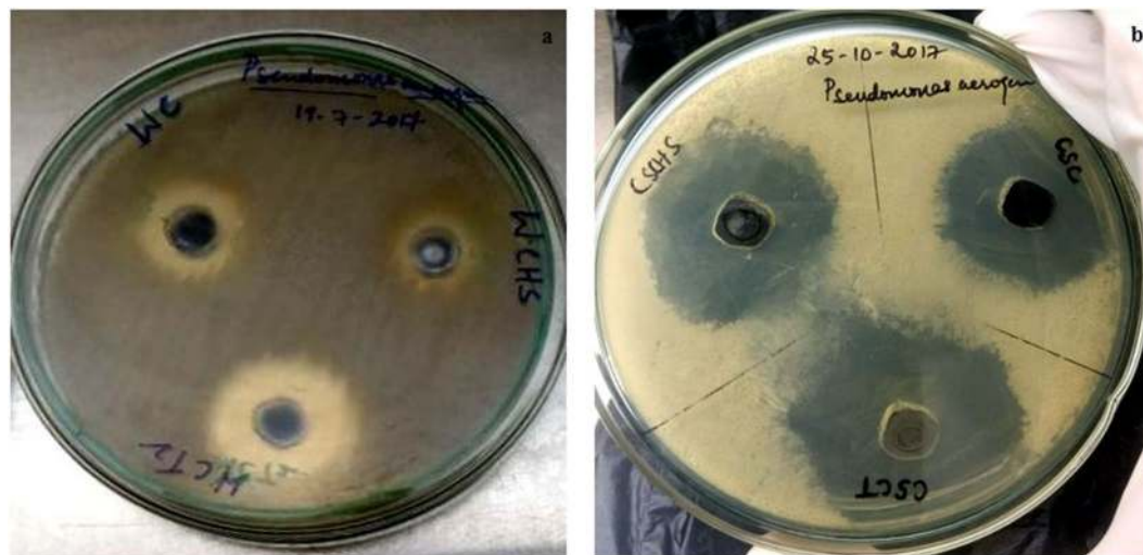
Figure 9. Photographs of the zone of inhibition produced by charcoal, GO and GTO nanocomposite derived from (a) wood and (b) coconut shell.
