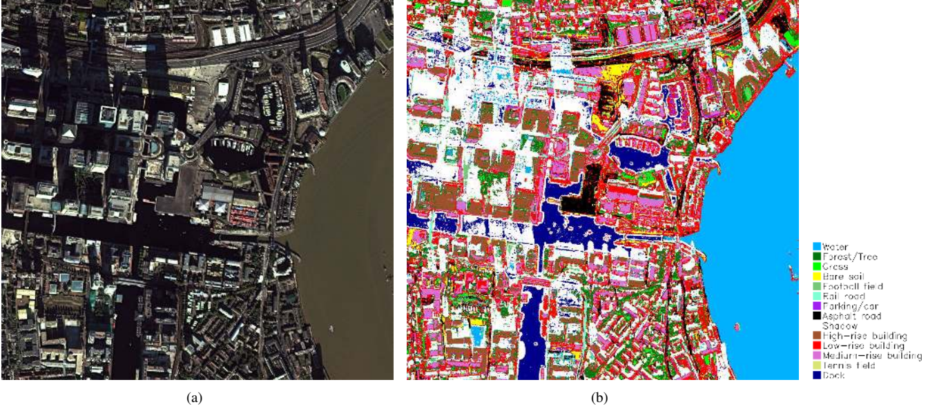
Fig. 3. Example of data fusion and classification (WV-2+Texture+DSM): (a) visible range multispectral image (bands 5,3,2), (b) FG fusion
