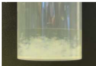
Figure 8. White precipitation in a 4.5 wt% Na-silicate solution containing 25 wt% SSW at 20 °C.
