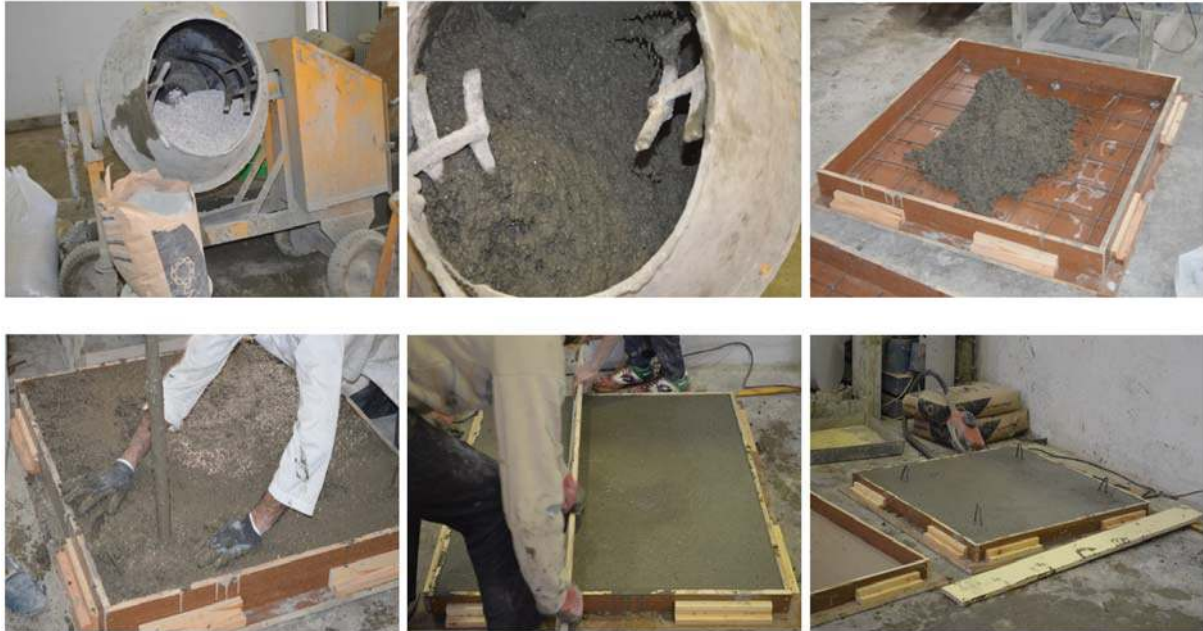
Figure 2: Mixing procedure of the tested two way slab
