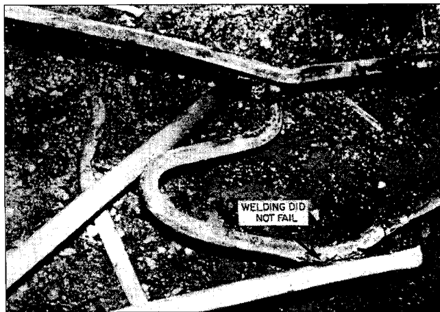
FIG. 12. Buckled Compression Diagonal (Kaminetzky 1991) (Reprinted by Permission)
