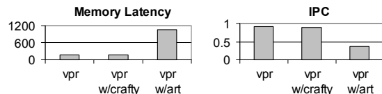
Figure 1: Memory latency and IPC for benchmark vpr when it is co-scheduled with crafty and with art
