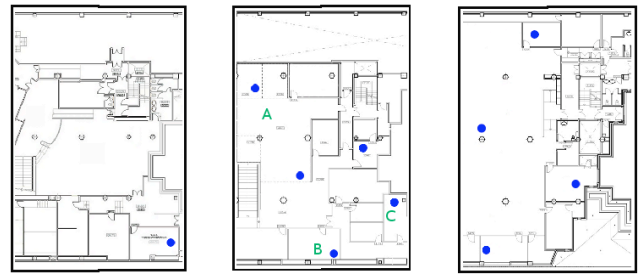
Figure 13: Testbed deployment. APs and stations have been deployed over 3 floors, ground floor (on the left), mezzanine (in the middle), and first floor (on the right). Each circle represents an AP, while stations are placed nearby the APs, one station per AP. Only stations A, B and C, relevant for some experiments, are shown in the map. Obstacles, as walls and desks are presented between all the AP links.
