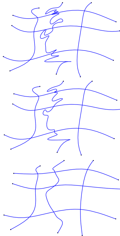
Figure 3: The faired wireframes with different \alpha : 10^{-1} , 10^{-3} , 10^{-5} (from top to bottom)
