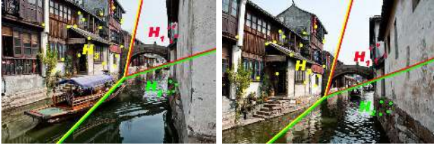
Fig. 4. Homography region partition. Matched points in the same cluster are marked in the same color. For each cluster, we fit a homography based on the matched points.
