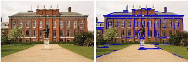
Fig. 3. Line detection. Blue lines show detected line segments whose length is at least 40 pixels.
