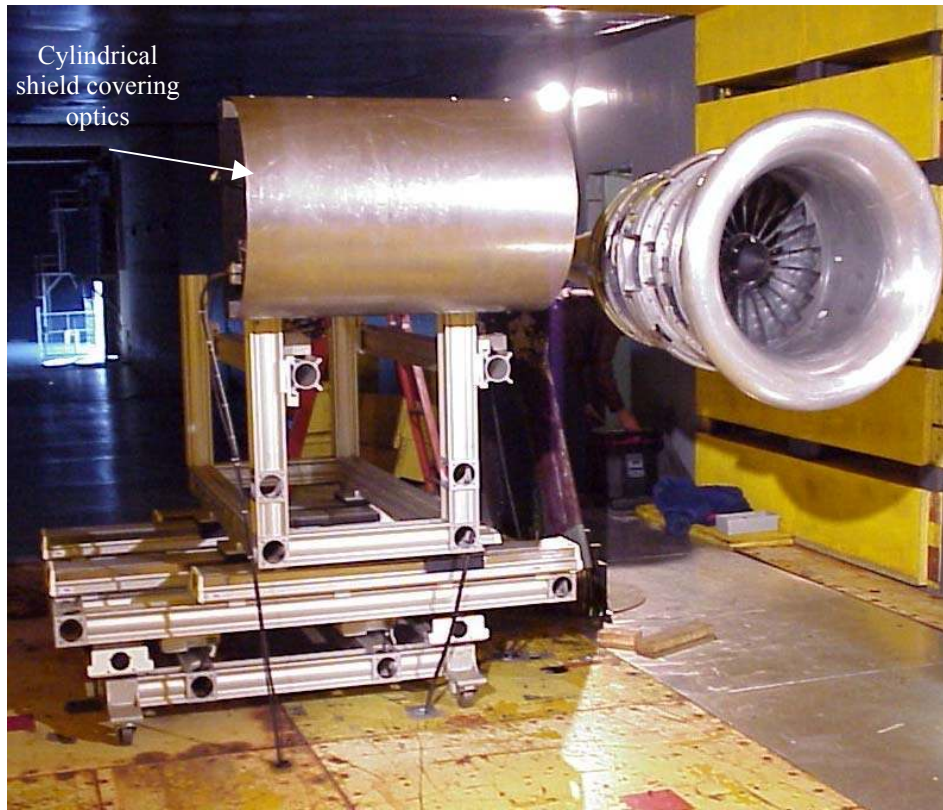
Figure 3. LDV system hardware installed next to the SDT model in the NASA Glenn 9 X 15 Foot Wind Tunnel.
