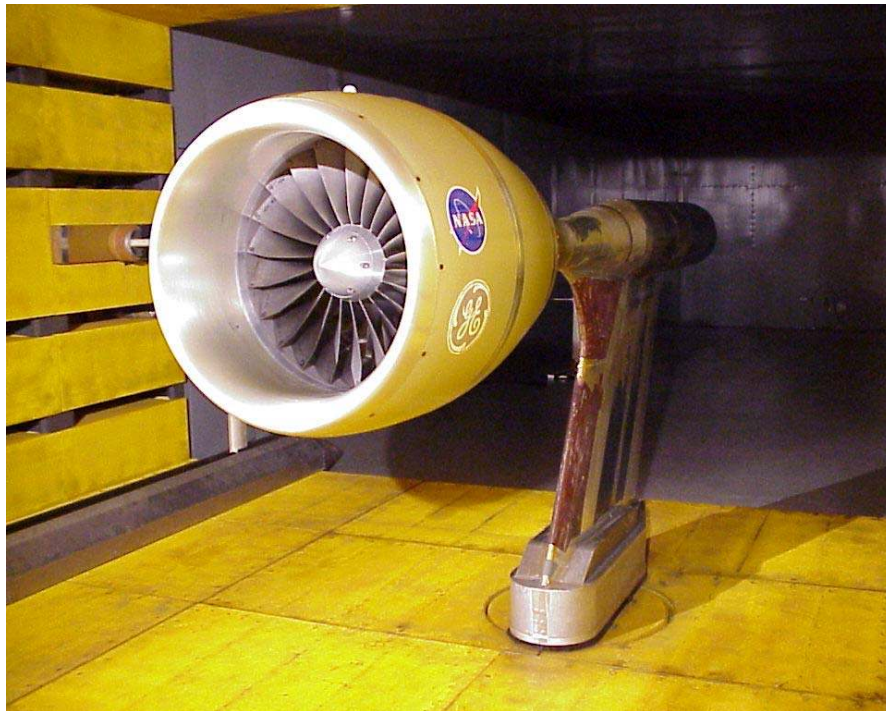
Figure 1. Source Diagnostic Test model installed in the NASA Glenn 9 X 15 Foot Wind Tunnel
