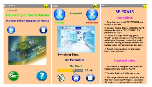
**Figure 25.** Mobile app for the RF power transfer system design. (**a**) Frontpage, (**b**) Timer set, and Bluetooth connection page, (**c**) Instruction page.
