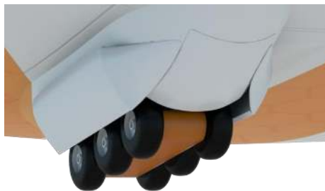
Fig. 12 Illustration of pod gear concept with toboggan.
