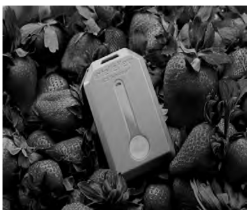
Fig. 2. Registration and reporting of temperature for shipments of perishable fresh fruit by using an RFID tag (label) Source: https://www.mhlnews.com/technology-automation/auto-id-getting-comfortable-rfid
