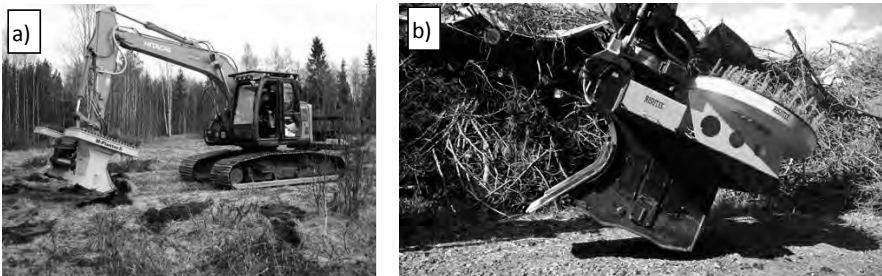
Fig. 2. Semi-automatic machines planting forest tree seedlings (a) M-Planter, and (b) Risutec.
