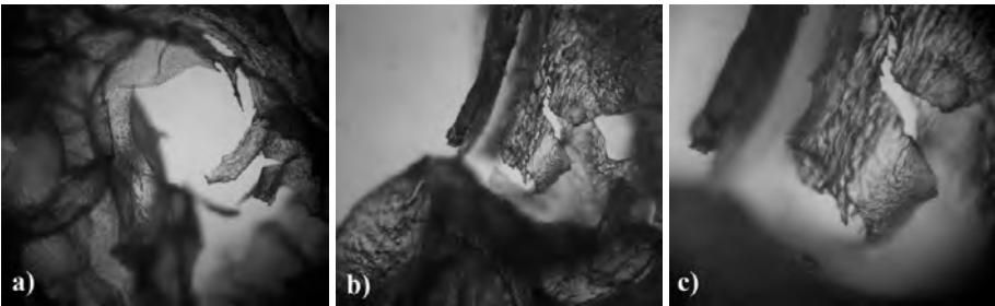
Fig. 4. Microstructure of potato starch-based foam materials without foaming agents (moisture content 17%, screw rotation speed 2.16 \text{ s}^{-1} ): a) zoom x40 b) zoom x100, c) zoom x200.
