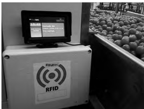
Fig. 1. Logistic management of fresh tomato stocks in sorting and storage using RFID technology, enabling error-free application of the FEFO method Source: https://espanol.rfidjournal.com/casos-de-estudio/vision?11485
