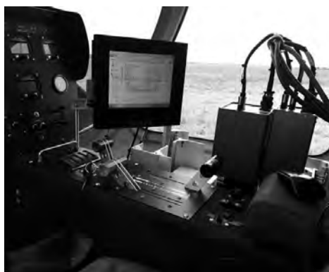
Fig. 2. Gyroplane cockpit with the remote sensing system.
