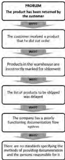
Fig. 3. 5WHY diagram analysing the cause of the problem related to the return of goods by the customer [author’s work]
