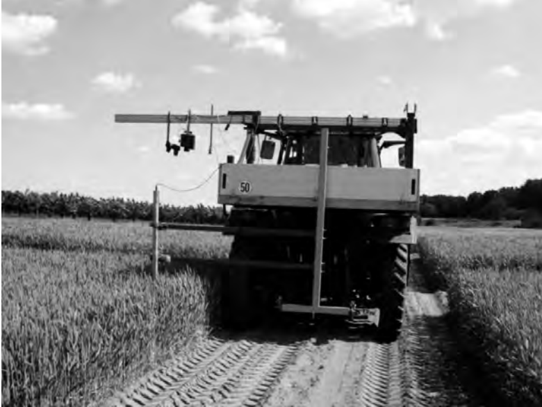
Fig. 1. Tractor with RGB camera, multispectral camera, ultrasonic sensor (from left to right on the gallows) and optoelectronic vertical sensor inside the crop canopy (left on the back three-point linkage) while test run
