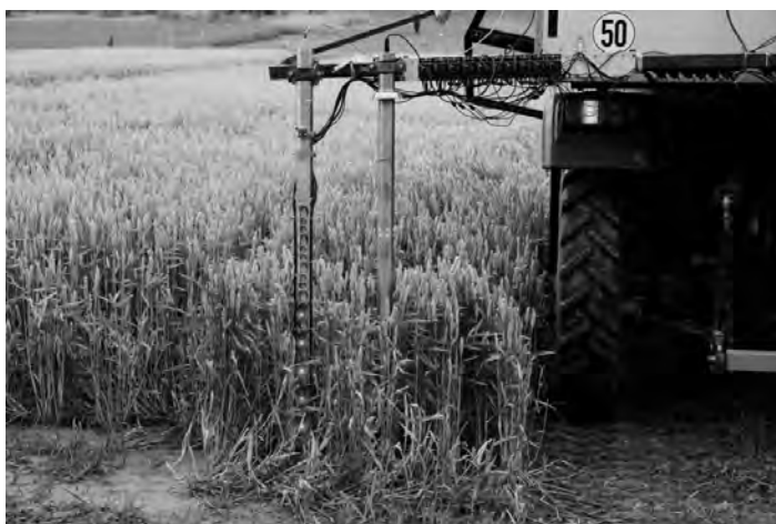
Fig. 5. Additional red and infrared LED-lighting at a vertical rod
