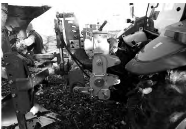
Fig. 3. Adjustable three-point hitch sensing dynamometer with a horizontal force capacity of 100 kN.
