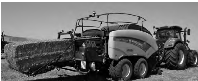
Fig. 2. Large square baler New Holland 1290 PLUS
