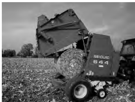
Fig. 1. The harvest of corn stover with the round baler New Holland 644.
