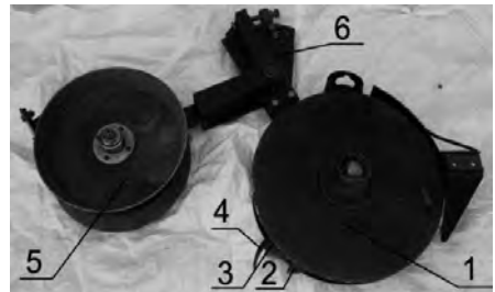
Fig. 2. A general view of the combined couler: 1 – disc; 2 – tip; 3 – seed drill tube; 4 – seed coverer (seed placer); 5 – packer roller; 6 – seed depth adjuster
