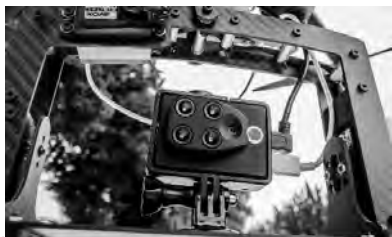
Fig. 1. Parrot Sequoia multispectral camera (source: authors)
