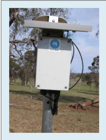
Figure 1. A soil sensor node on Kirby Farm near Armidale, New South Wales, Australia. The node is powered by a solar panel on top. A strong post keeps the electronics above any livestock, while carrying a wire to the sensors embedded in the soil a metre to the side.
