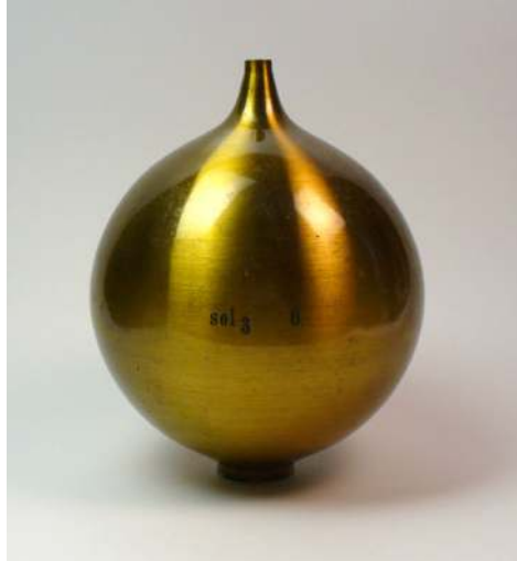
Figure 2.2: A brass Helmholtz resonator, from Max Kohl made around 1890-1900. Photograph by user brian0918, www.wikipedia.org .
