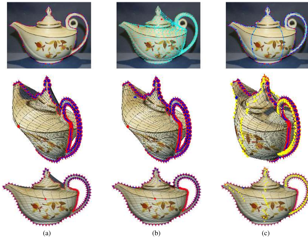
Figure 3: Steps in model building for a genus one surface. (a) User supplies silhouettes and marks points of high curvature. Some of the model spills into the background. (b) User drags model points into the interior of the object. The minimization corrects the spill while maintaining silhouette consistency. (c) The user adds inflation curves to improve the 3D shape, creating a narrower spout, and adding a bulge at the base. Overall user input is the silhouette (power-assisted), three spillage drags, and six inflation curves, none of which need to be precise. Middle and Bottom row: 3D models with the (u, v) curves and constraints.
