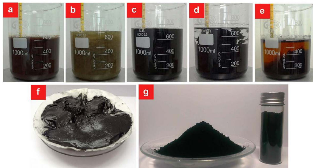
Figure 1. Consecutive steps of ARGO production. a oxidation and exfoliation of graphite in the presence of oxidizing agents. b reduction and conversion of insoluble manganese ions to soluble ions by addition of ascorbic acid. c changing the color of exfoliated graphite oxide from greenish yellow to black at the early stages of reduction. d loss of the hydrophilicity of GO by pausing the stirring. e precipitation of ARGO after accomplishment of the reduction stage and cooling down to room temperature. f easy filtration of ARGO by conventional cellulose filter paper. g attaining ARGO in the powder form after freeze drying.
