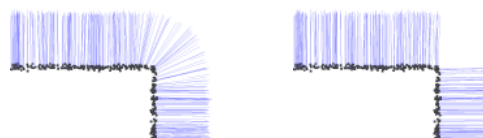
Figure 1: Reconstructed normals of a corner with Least Square Regression (left) and our method (right).
