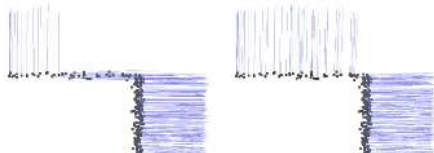
Figure 3: Reconstructed normals of a corner with sharp density variation: Li et al.'s algorithm (left) and ours (right).
