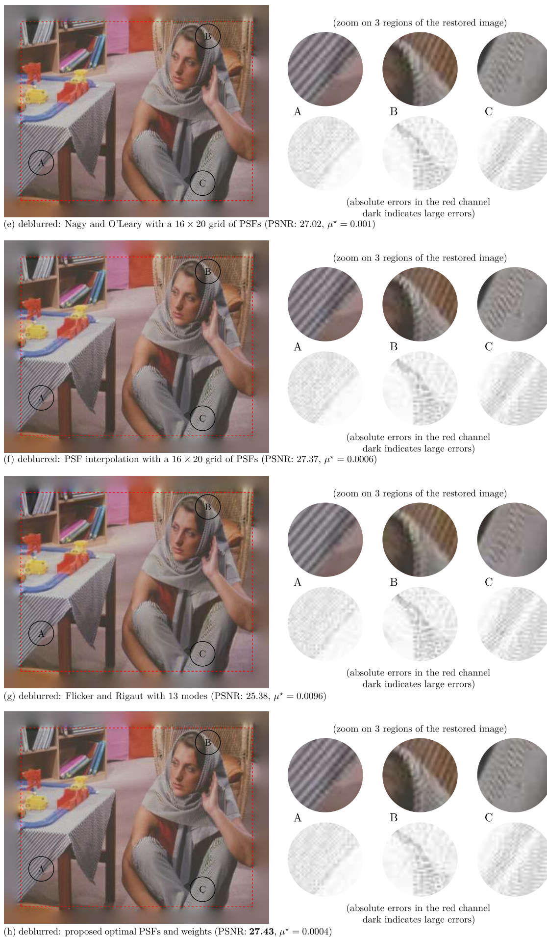
Fig. 9 (cont.) Restoration of a color image degraded by chromatic and shift-variant blur: (e-h) deblurring with shift-variant PSF models of comparable computational complexity (fine models).
