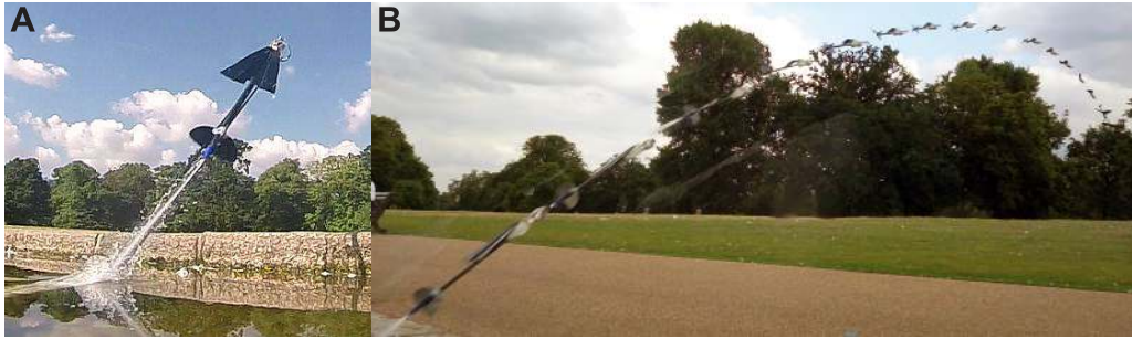
Fig. 1: Outdoor testing of the presented prototype: An AquaMAV can return water samples and data from isolated areas of water, using a powerful burst of water jet thrust to accelerate free of the water and transition to flight. A: The AquaMAV launches itself out of water. B: Timelapse of a launch trajectory. Wings are deployed in the final snapshot.
